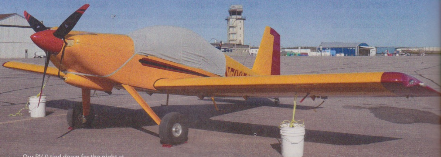
Our RV-9 tied down for the night at Inuvik. The tie-downs are buckets of concrete, presumably for use in snow.
