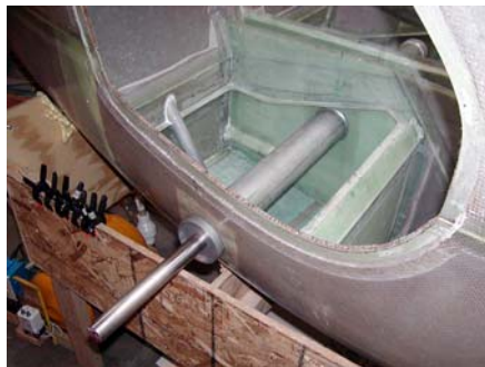
Wing Tube Jig in place—note fuel fill tube
