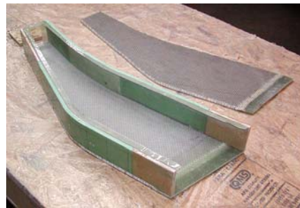
Rotor Tower partial assembly before closeout—note pre-fabbed flanges for closeout
