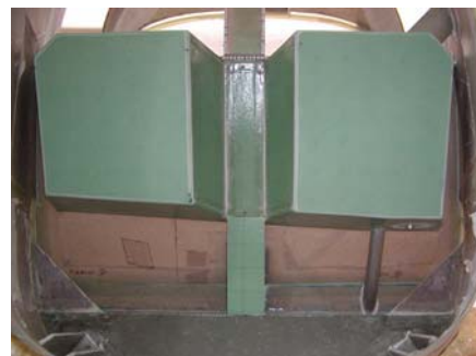
Header Tank Detail—fill tube lower right & fuel line attachment fitting
